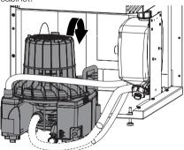
Connect the suction hose and discharge hose to the suction unit.
