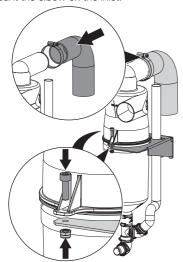
Attach the condensation separator with the holder to the unit and secure.
