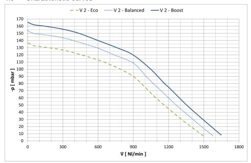
Fig. 2: Characteristic curves for: 7177-01, measured in accordance with ISO 10637
