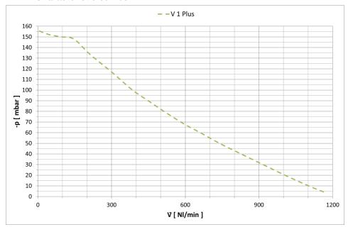
Fig. 1: Characteristic curves for: 7182100200, measured in accordance with ISO 10637
