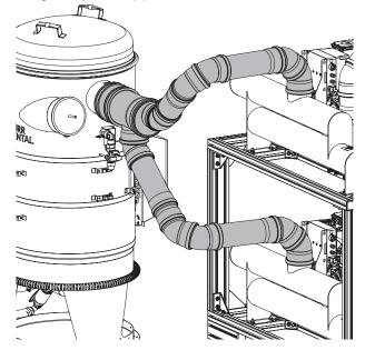
> Route the suction pipes from the in-house installation to the central separation unit and push them onto the suction connections.
