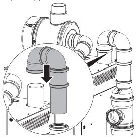
**10.** Using DürrConnect parts, connect the condensate waste water hose to the waste water system of the condensation separator.
