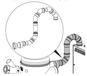
8. Route the suction pipe from the in-house installation to the central separation tank and push it onto the suction connection.
