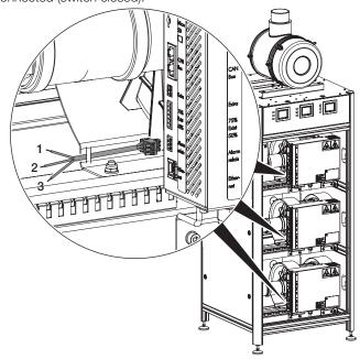
Alarm connection circuit diagram
