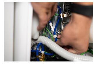
Plug thin green tube from dentist's panel side to distilled water bottle connection (2,5 bar).
