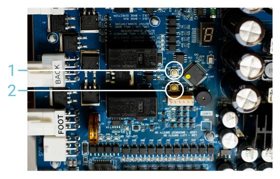
Chair and backrest movements are controlled using buttons 1 and 2.
