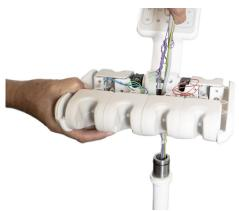
Secure the control panel with lock ring.
