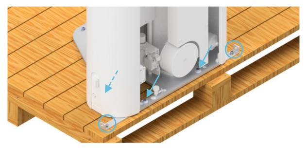
Fix the unit base in eight points (all arrows). Use dowels, washers and screws from accessories as shown at the picture.
