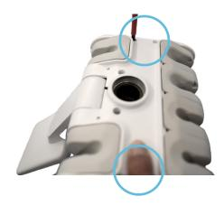
Pass the cable harness through the hole. Then put on control panel at arm.
