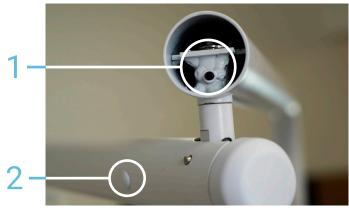
Install brake of the rotating part of the light arm. Insert elements into the hole, as it's shown at the picture, screw in, fit the esthetic cover.
