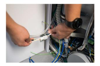
Plug blue tube from dentist's panel side to blue tube from main air filter regulator (4 bar).
