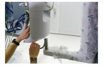
Secure the arm with secure ring (1). Use brake screw as needed (2).
