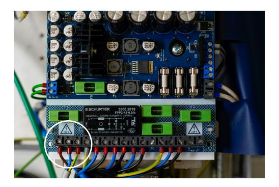
For installation purposes, before the safety switch from the assistant's arm is connected to chair electronics PCB, you can use a jumper to connect the 2 pins marked "SAFE ASSIS" to have all 4 blue LED lights and be able to move the chair in all directions.
