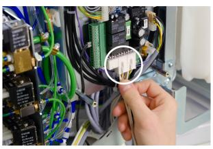
Plug blue tube from dentist's panel side to blue tube from main air filter regulator (4 bar).
