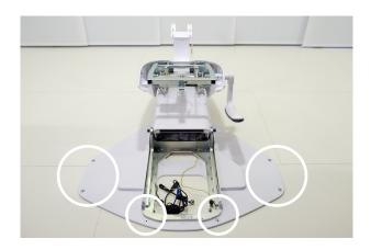
Remove powerblock from it's package and place it in powerblock area.
