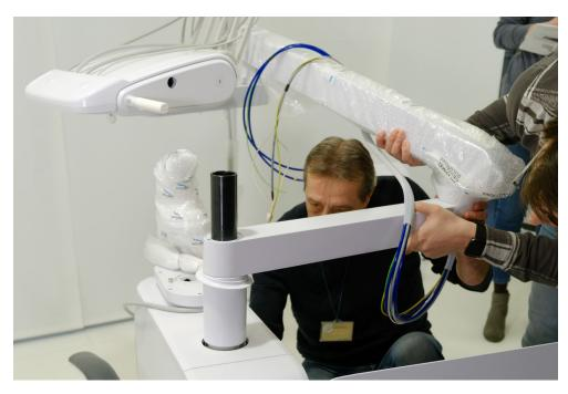
Put the metal bar inside post, find the correct position.
