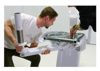
After putting cuspidor block holder in the place, first screw bolts (1), then screw bolts in back (2).
