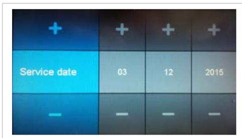
The "Service Date" service menu displays the due date of the next service check. Once a service check is completed, the date for the next service check can be set. KaVo recommends performing the service check every two years together with the safety check.
