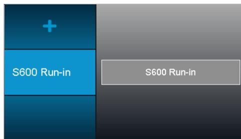
After replacement of the ball bearings of the S600 LED handpiece, the "S600 run-in function" is available in the "S600 run-in" service menu to attain uniform distribution of the grease, reduction of the idle power/temperature and a smooth running performance.
