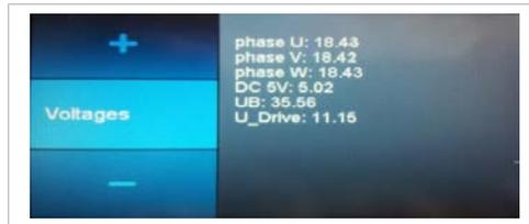
The "Voltages" service menu displays the phase voltages of the motor. The phase voltages must be distributed evenly. No clearly higher or lower voltage must be applied to any of the phases.
