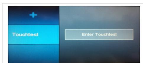
Errors related to touch input can be checked with the touch analysis in the "Touch test" service menu. For this purpose, touch the display surface or draw lines and compare the actual position to the position displayed by the device. If the position deviates too strongly or if there are jumps, the control panel needs to be replaced.
