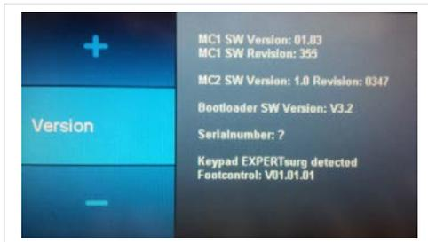
The "Version" service menu displays information about the unit such as the software and hardware version and the boot loader used.
