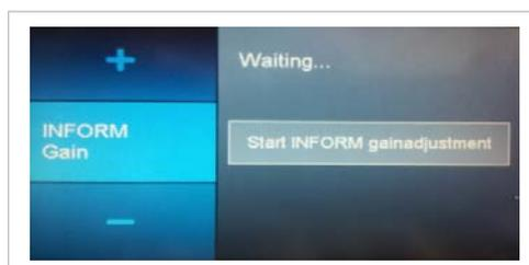
The "INFORM Gain" service menu can be used to start the calibration of the motor electronics. The motor runs briefly and stutters while this is done.
