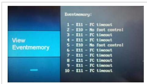
The "View Eventmemory" service menu displays the 10 most recently saved error messages. The error with the lowest number is the most recent error.
