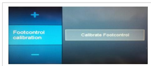
After replacing the control button of the foot control, the electronics can be re-calibrated in the "Foot control calibration" service menu.
