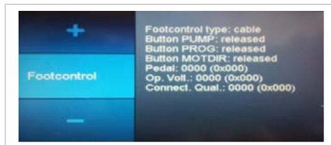
The "Footcontrol" service menu can be used to test the keys/potentiometer in the foot control. Actuation of a foot control key must be indicated by a corresponding response on the display. The potentiometer value shown must be between 0 (not actuated) and 1000 (full deflection).
