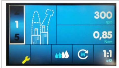
The "torque test control unit" (Mat. no. 1.005.0608) is used to check for torque.
