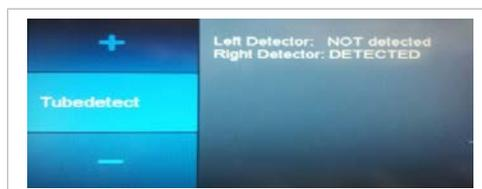
The "Tubedetect" service menu can be used to test the detection sensors for the coolant hose or the coolant hoses. The sensors are situated on the board. Upon connecting a hose, the hose needs to be displayed as "detected".
