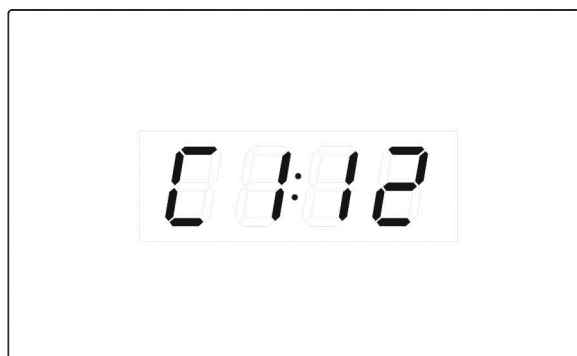
fig. 29 – Cloc parameters. Hold down the Start/Stop button to access the parameters, in this case identified as C1 , C2 , etc. Parameter C1 sets the current year, C2 the month, etc. Use the Selection buttons to modify the parameter. Use the “ Functions ” button to move to another parameter. Confirm changes using the Start/Stop button.
