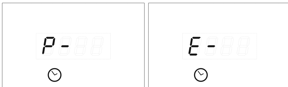
fig. 23 – RESET: during the RESET the display shows "P- ". At the end of the RESET cycle, "E- " appears on the display.
