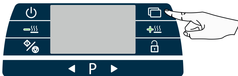
fig. 9 – “Functions” button With the cycle in progress or being selected, pressing the Functions button displays the parameters of the wash cycle: A0 value, Temperature and Time Remaining.
