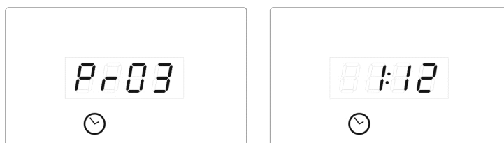
fig. 19 – Once the cycle start command is given, the display alternates the program selected with the time remaining before it actually starts.
