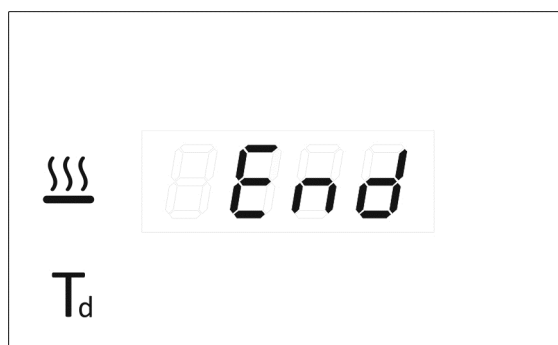
fig. 15 – End of cycle, display screen. The word End indicates that the washing process has been completed correctly.
