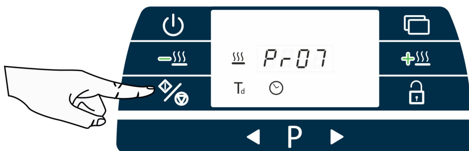
fig. 16 – Interrupting a Program: hold down the Start/Stop button
