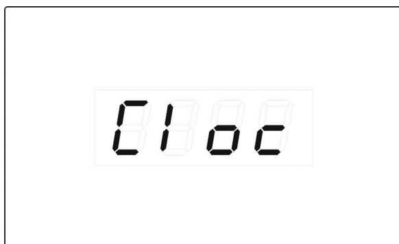
fig. 29 – Cloc parameters. Hold down the Start/Stop button to access the parameters, in this case identified as C1 , C2 , etc. Parameter C1 sets the current year, C2 the month, etc. Use the Selection buttons to modify the parameter. Use the “ Functions ” button to move to another parameter. Confirm changes using the Start/Stop button.
