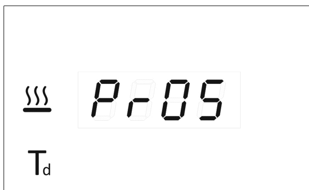
fig. 11 – Example of a Display screen. Program 5 selected The program includes a drying phase – Drying LED on. The program includes a thermal disinfection phase– “Td” LED on.
