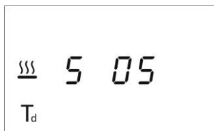
fig. 3 – If a cycle is interrupted the appliance switches to Suspension mode. e.g. Display screen, Suspension of program 5: “S 05”.
