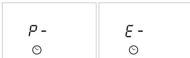
fig. 4 – RESET: during the RESET the display shows “P-”. At the end of the RESET cycle, “E-” appears on the display.
