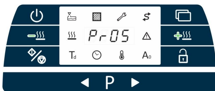
fig. 1 – Control panel: digit area in the centre with indicator LEDs around the perimeter
