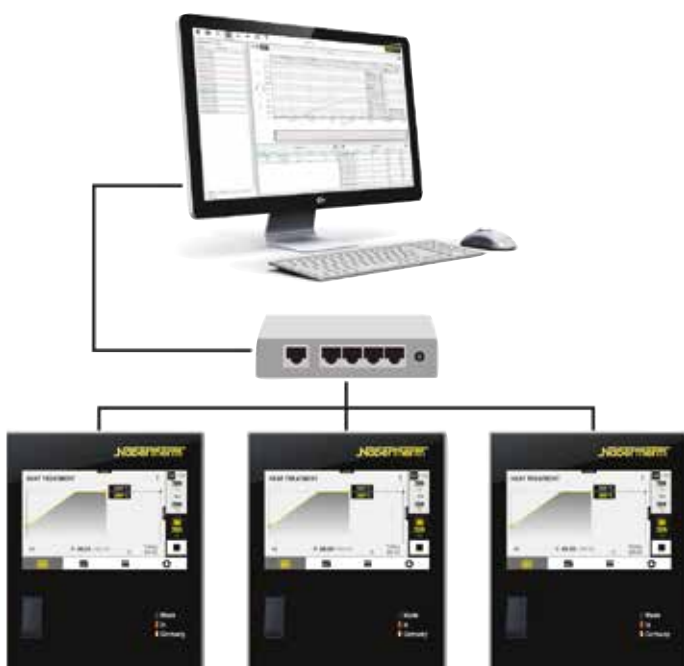
Example lay-out with 3 furnaces
