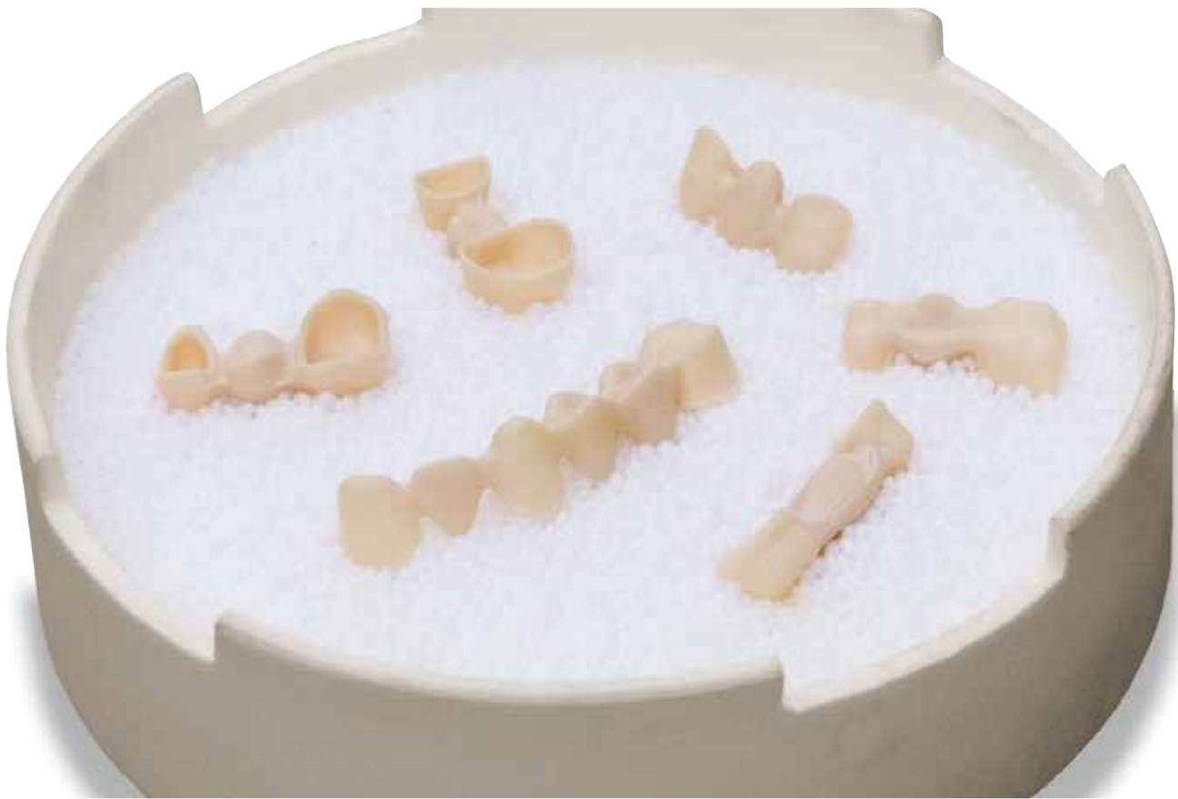
Charge Saggar for Sintering Furnaces LHT 01/17 LB Speed, LHTCT 01/16, LHTCT 03/16 and LHT 01/17 D
