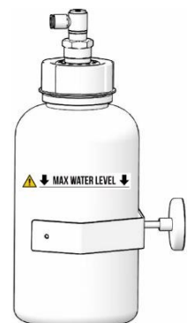
Fig. 10: Check of the condensate collection vessel
