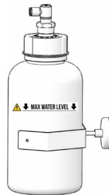
Fig. 18: Check of condensate collection vessel
