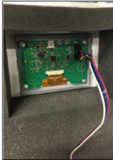
Fig. 17: Connecting the display connector
