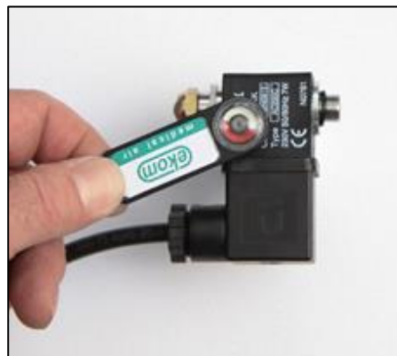
Fig. 19: Check of solenoid valve operation
