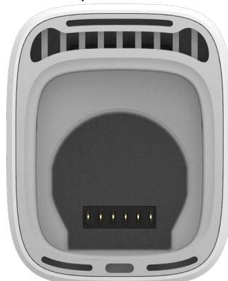
Figure 1 : Contact points on scanner handpiece
