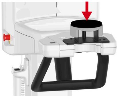
3. Place the dental cast on the holder as shown on the GUI.
