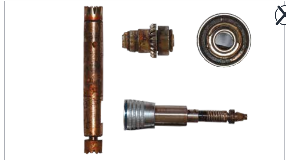
Improperly serviced handpieces
