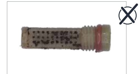
Water filter is clogged and / or dirty
