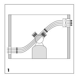
The room temperature must not be allowed to fall below 10 °C otherwise a trouble-free operation of the control unit within the machine cannot be guaranteed. If room temperatures exceed 40 °C, additional ventilation must be provided by installing a fan (see Fig. 1).
